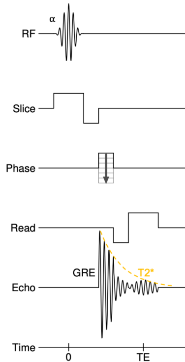
Figure 2.2: Sequence diagram of a simple gradient echo experiment. The gradient echo signal arising at TE is induced by a prior de- and rephasing gradient.
