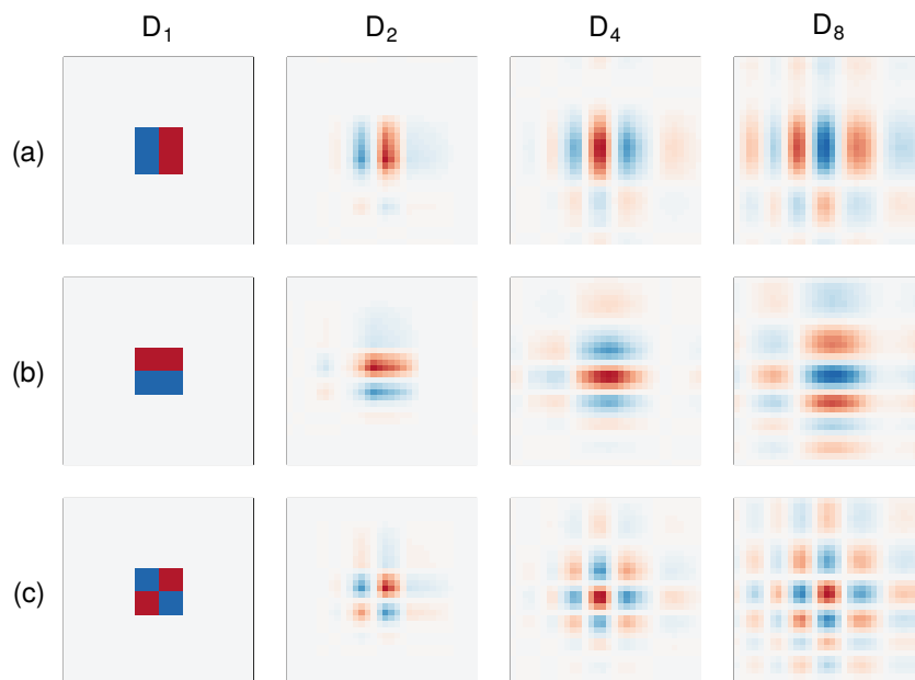
Figure 2.7: Vertical (a), horizontal (b) and diagonal (c) daughters corresponding to the Daubechies wavelets from figure 2.5. Negative values are shown in blue, positive in red.
