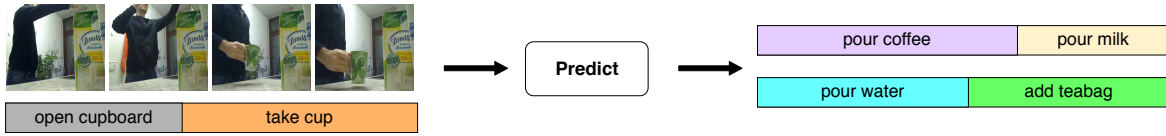
Figure 7.1: The anticipation task. Given an observed part of a video, we want to predict the future activities that might follow in the future with their durations. The model outputs a collection of samples to represent the uncertainty in the future actions.
