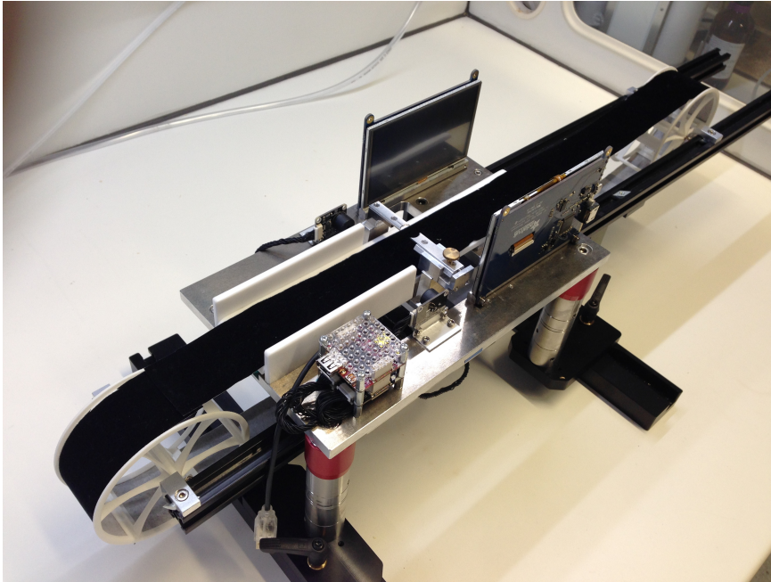
Figure 2.4.2: A prototype of the customized horizontal treadmill with the belt - The horizontal treadmill was mounted on two sliding bars, compatible to the rails under the two-photon microscope in order to be moved back and forth for convenience (the two large black bars). The bright black velvet fabric slid on a Teflon plate and two 3D printed wheels. Wheels were attached to the treadmill with shafts. A microprocessor collected the data and delivered stimulus commands.
