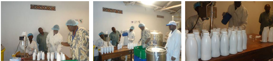
Figure 11: The process of hot filling of Mamera Source: Tukahirwa et al. (2013)
